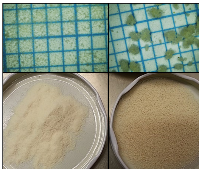
Figure 1. Uncoated powder (left images) and coated granular (right images) forms of the LBXG can be seen. The size of each square is 1000 µm in the upper images. The LBXG powder is in the range of about 10-20 µm, while the coated granular LBXG is in the range of 100-1000 µm (750 µm on average).
